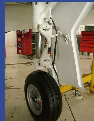
TBM Landing Gear.
