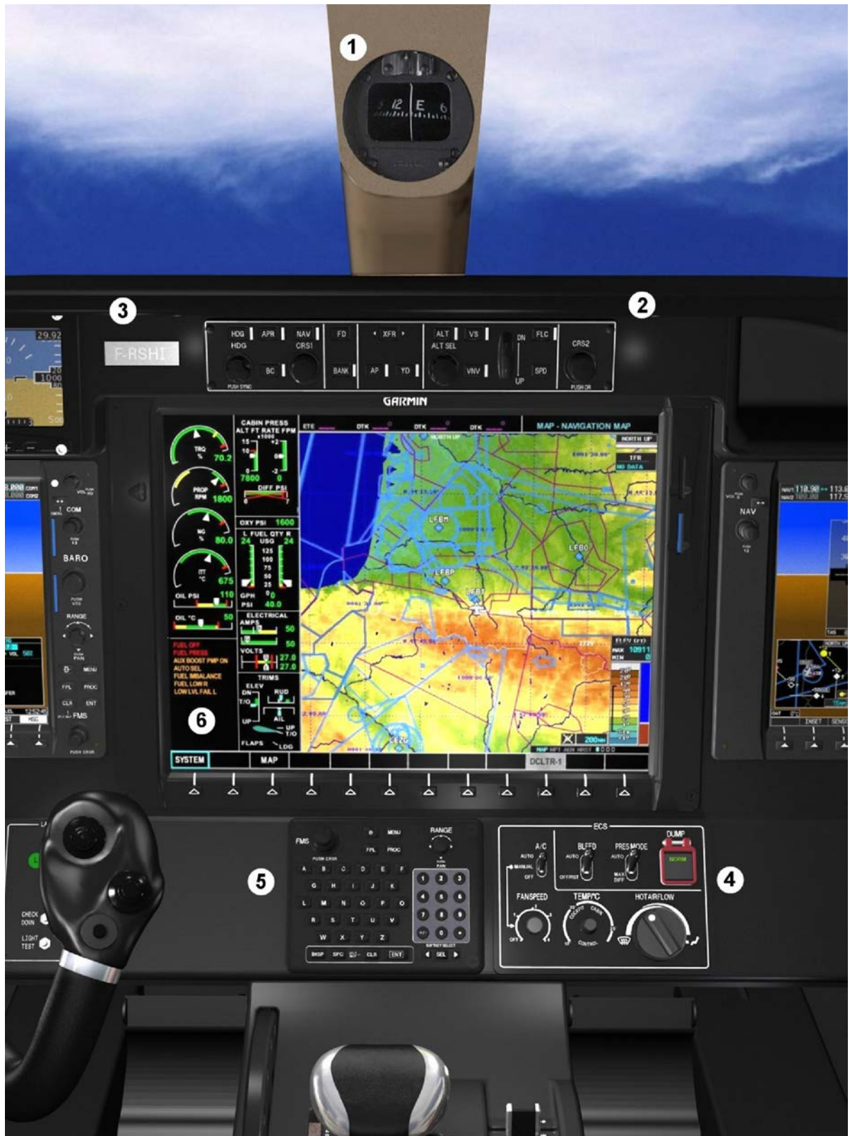
Figure 7.3.4 (2/2) - CENTRAL INSTRUMENT PANEL (Typical arrangement)
