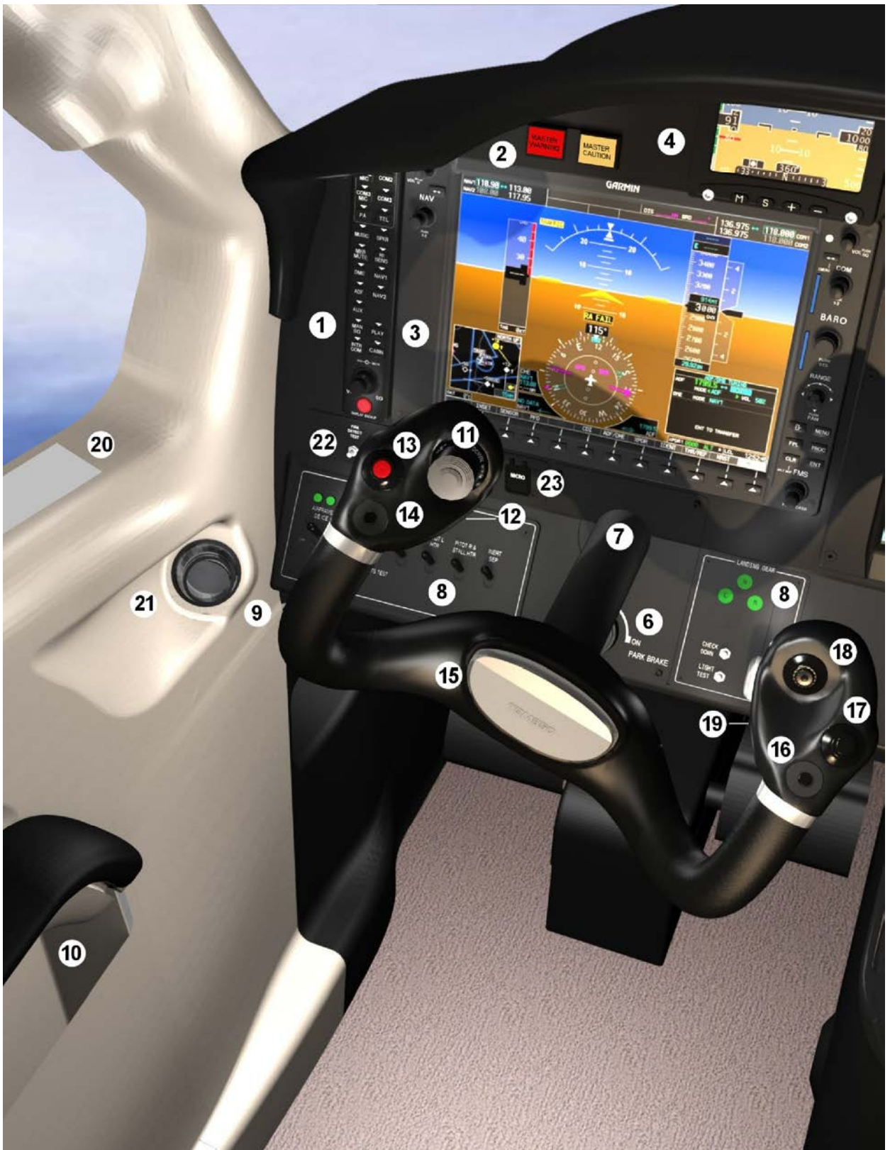
Figure 7.3.3 (2/2) - LEFT INSTRUMENT PANEL (Typical arrangement)
